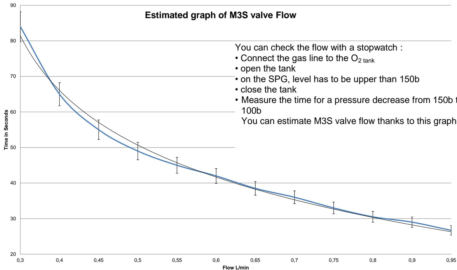
You can check the flow with a stopwatch :
