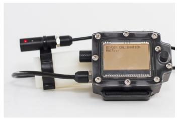
As soon as calibration is done, MONOX displays the result for each cell and their voltage. Then go to Save and Exit
