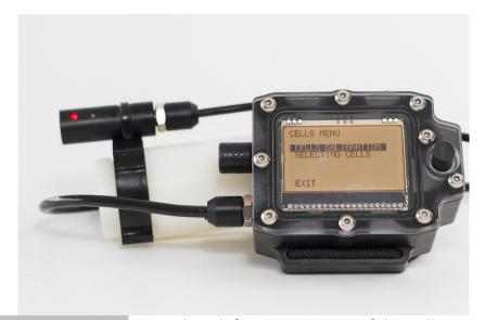
SELECTING CELLS is used to define parameters of the cells : to choose the cells type and their number. With TRITON, the by default values are as follows : generic type and 3 cells.
