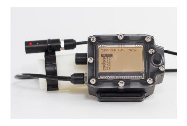
TRESHOLD is used to select the range of treshold.
