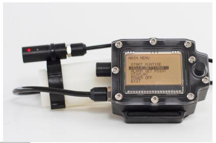
Start runtime is used to start the calculation of the average (when the average display is activated)
