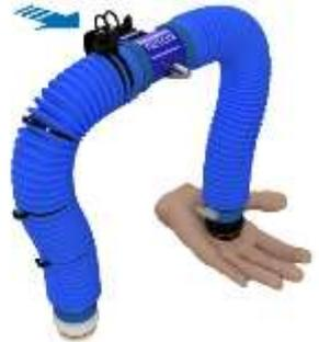
FIGURE 3.15 – Loop assembly overpressure test.
