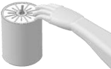
FIGURE 3.4 – Set up of the grid on the canister scrubber
