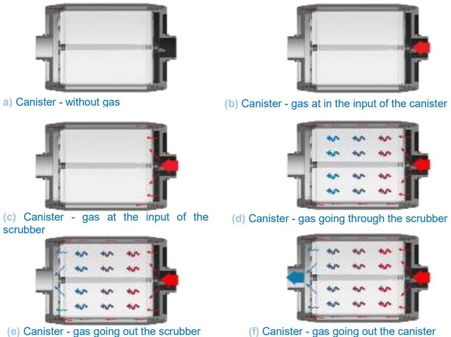
FIGURE 2.4 – Canister operation
