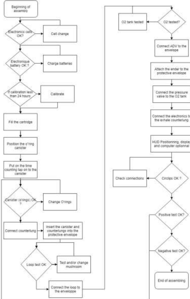
FIGURE 3.22 – Flow chart of the tests to be undertaken on the TRITON® before each dive.
