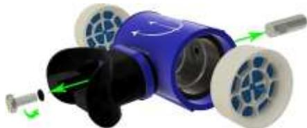
FIGURE 4.4 – Dissambling of the DSV from the loop.
