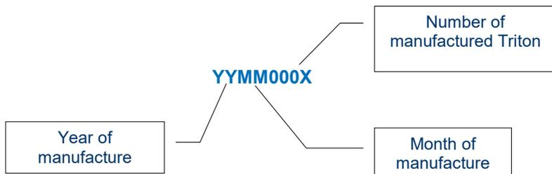
**FIGURE 2.7 – Serial number explanation**
