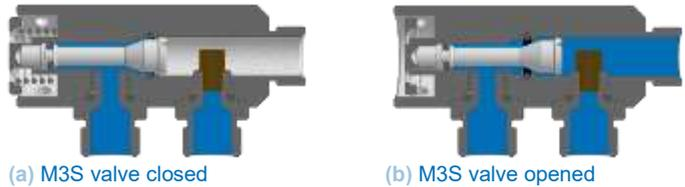
Opened valve, the diver activates the valve push button enabling the addition of oxygen (cf. figure 2.5.b). In its closed position, the flow automatically returns to 0,7L/min. (cf. figure 2.5.a).
