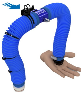
FIGURE 3.15 – Montage boucle test surpression.
